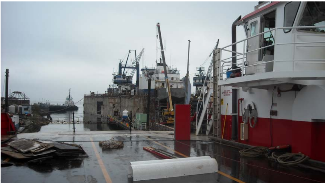
View of the busy Vigor Marine shipyard from the deck of the Charlie Wells. The refrigeration ship in the background has been cut in half, adding 40 feet to the center section, and 20 feet in length at one end. Amazing!
