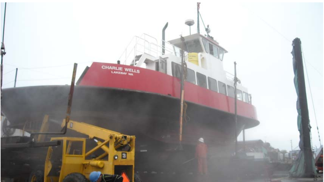
Vigor Marine personnel cleaning the hull on Tuesday morning.
